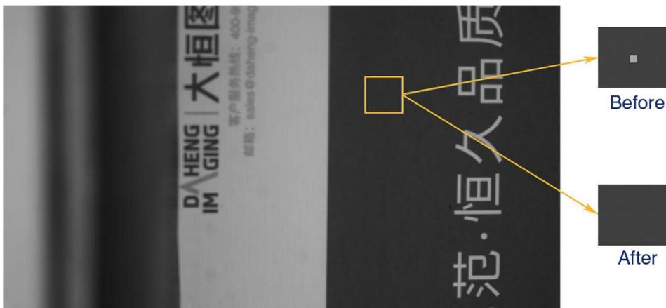
Figure 8-60 Defect pixel correction effect in actual scenario
